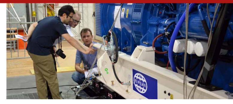
demonstrate reliability and performance after the seismic test, the generator sets were then returned to FG Wilson's UK facility in Larne, which houses Europe's largest testing and development facility for generator sets, built at a total investment of \$26 million.
